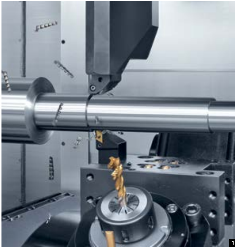
1: Main spindle with 6,000 min -1 , or optional strengthened model rated with 5,000 min -1 2: 6 sided complete machining due to counter spindle (option) with 6,000 min -1
