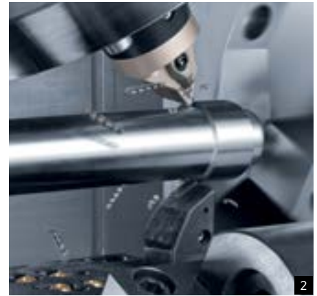
1: Main spindle with 6,000 min -1 , or optional strengthened model rated with 5,000 min -1 2: 6 sided complete machining due to counter spindle (option) with 6,000 min -1
